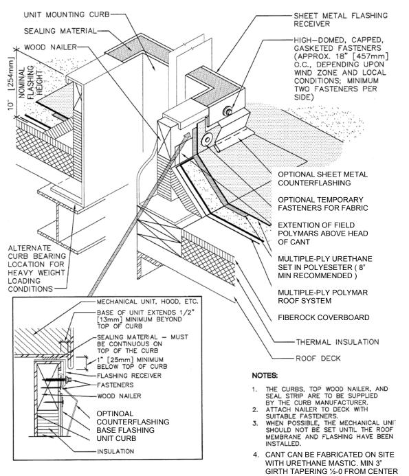
ADUREL POLYMAR ROOFING SYSTEMS **CURB DETAIL**
